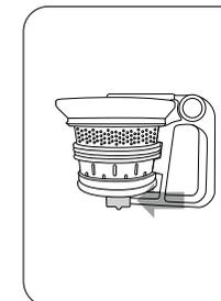
In that state, push the slide rock at the bottom with the strainer and tighten it.
