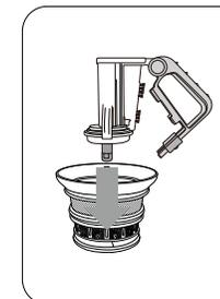
After inserting the fastening bar into the silicon ring groove in the center of the strainer, then lower the handle.
