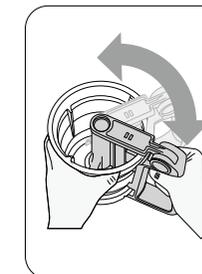
Wash from side to side while rotating the dual cleaning tool and strainer in opposite directions under running water.
