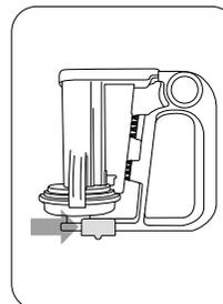
Push the slide lock of the dual cleaning tool toward the handle to release it.
