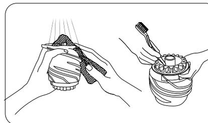
Remove foreign substances (seeds, grains) stuck in the screw groove with the tip of the cleaning brush.
