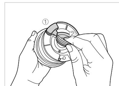
The silicon cover is removable for cleaning. After cleaning, place the silicon cover in regular sequence on as shown in the picture.
