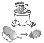
If leafy ingredients wrap around the juicing screw, open the lid and remove the fibers before continue juicing.
