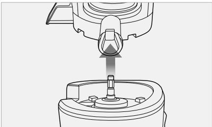
**4** Remove the juicing screw, strainer and rotation wiper unit from the juicing bowl. Clean with provided brush.
