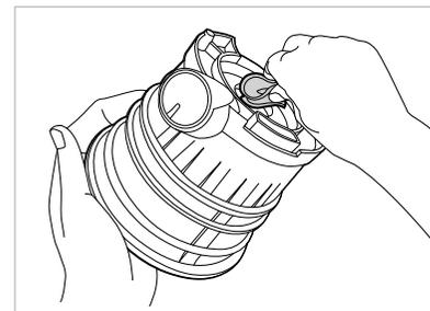
The silicon ring is removable for cleaning. After cleaning, place the silicon ring on as shown in the picture.
