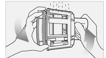
**3** Thoroughly rinse the inside and outside of the strainer under running water.
