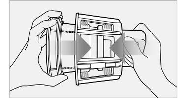
**2** Under running water, rotate the cleaning tool and the strainer in opposite directions to clean.
